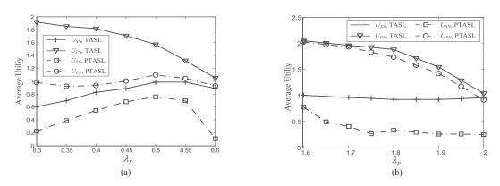
Fig. 6. The average utilities of SN and PN, i.e.,  $U_{SN}$  and  $U_{PN}$ , are depicted in terms of (a) the average generation rate of SPs, i.e.,  $\lambda_S$ , and (b) the average generation rate of PPs, i.e.,  $\lambda_P$ , where p = 1.
