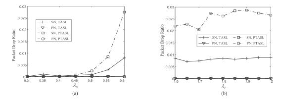
Fig. 9. The packet drop ratios of SN and PN are depicted in terms of (a)  $\lambda_S$  and (b)  $\lambda_P$ , where p = 1.
