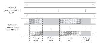
Fig. 1. In the proposed traffic-adaptive spectrum leasing (TASL) scheme, the infinite time of the  $N_S$  licensed channels leased from the PN to the SN are synchronously divided into leasing and buffering periods with variable time lengths, which can fully adapt to the real-time secondary traffic.
