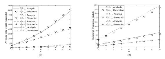
Fig. 4. (a) The expected buffering time for all SPs or PPs in one leasing or buffering period versus *n*. (b) The expected number of SPs or PPs transmitted in one leasing or buffering period versus *n*.
