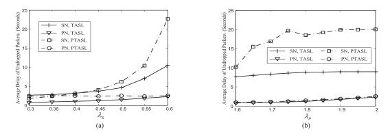
Fig. 8. The average delays of undropped SPs and PPs are depicted in terms of (a)  $\lambda_S$  and (b)  $\lambda_P$ , where p = 1.
