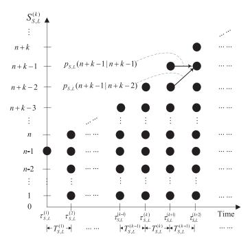
Fig. 10. Possible number of buffering and transmitting SPs seen by one SP newly generated in a leasing period, where each black circle denotes one possible number.
