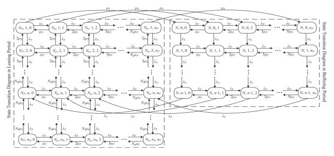
Fig. 2. State transition diagram of the Markov chain  $\{CH_t, SP_t, PP_t\}$ .
